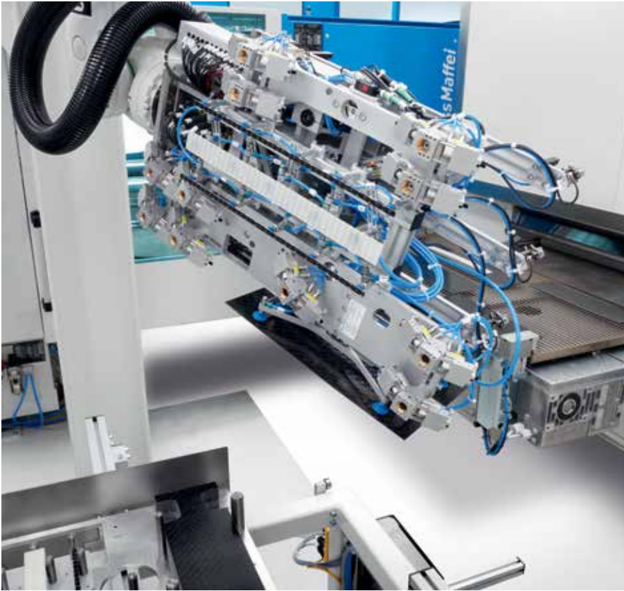
Complex multifunction gripper for inserting, moving and demolding parts.
