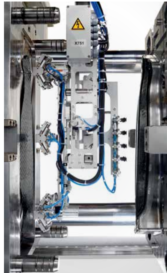
Fully automatic handling of semifinished product and complete part
